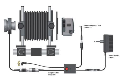
Schneider electronic shutter connections
